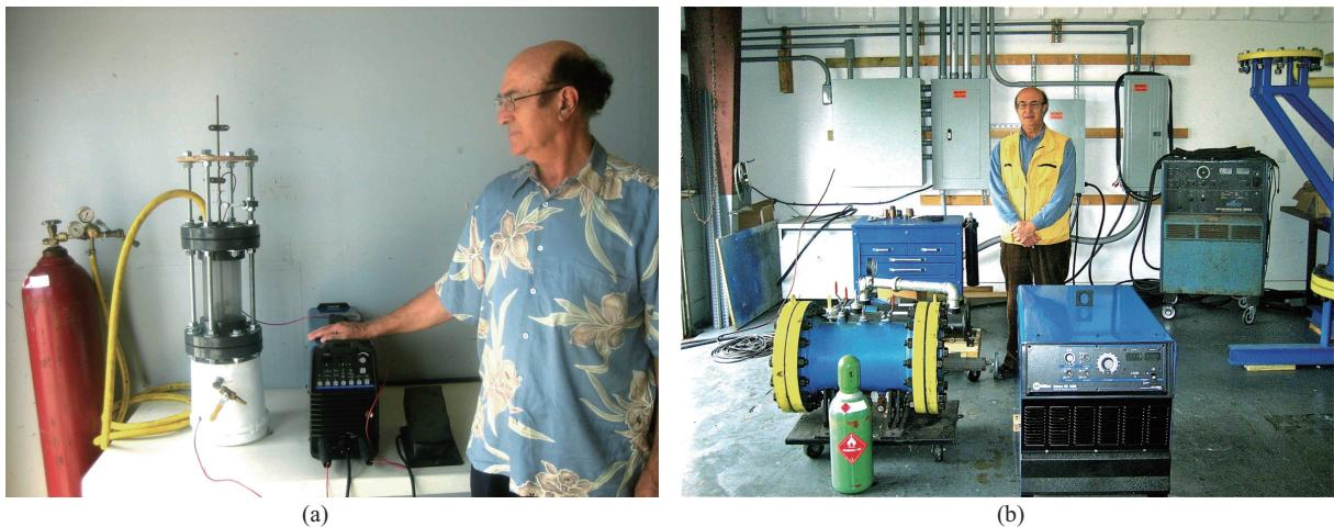
Fig. 3. A picture in the left of the first reactor in translucent PCV used in tests [9] with the hydrogen gas at 15 psi (Fig. 3a), and a view in the right of the second reactor built with schedule 40 steel used in tests [9] with the hydrogen gas at 100 psi.
